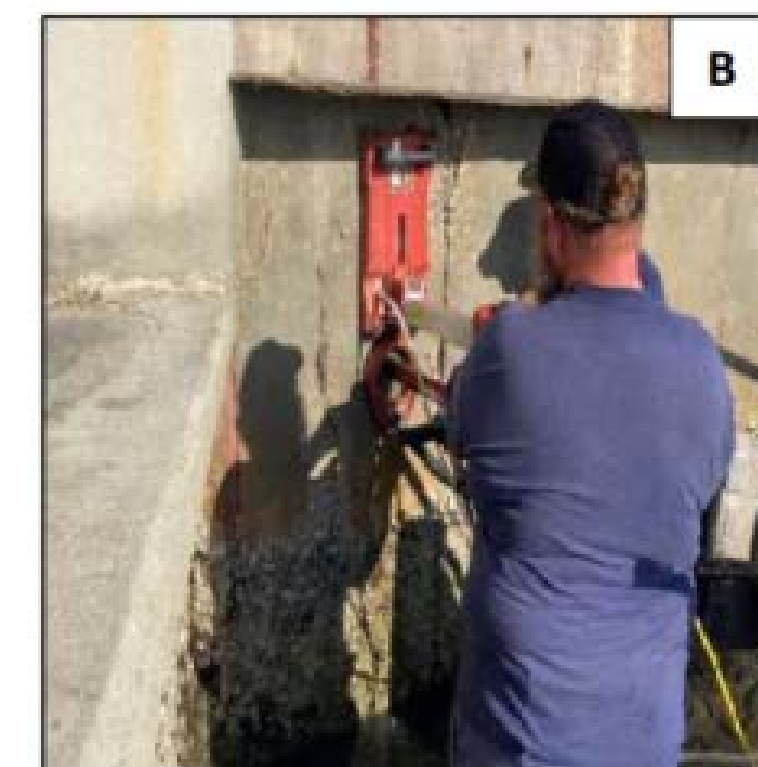
Figure 1: Crack inspection, drilling cores, and rebar inspection. A) Evident corrosion product at the bottom of the core; B) Core extraction; and C) Delamination at the level of the steel rebar.
