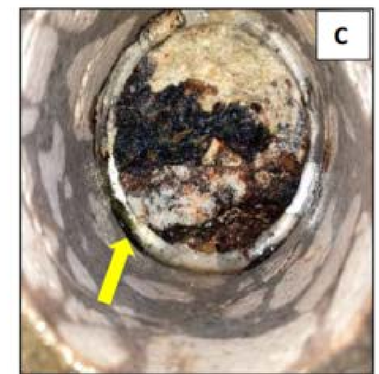
Figure 1: Crack inspection, drilling cores, and rebar inspection. A) Evident corrosion product at the bottom of the core; B) Core extraction; and C) Delamination at the level of the steel rebar.
